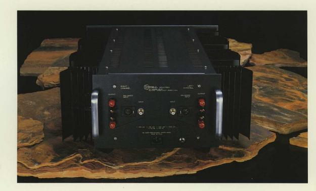
The KSA-150 and KSA-250 bave balanced inputs via XLR connectors and single-ended inputs via RCA connectors. There are two sets of 5-way binding posts per channel to allow easy speaker bi-wiring.
